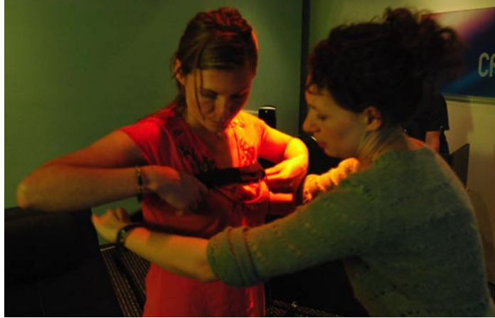
Attaching the breath sensor belt around the participants. The sensor measures breath related changes at the point of contact. Most participants can obtain good readings with the sensor attached just above or below their breast area.
